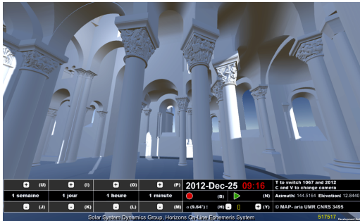
Figure 8: Desktop implementation of the digital heliodon.
