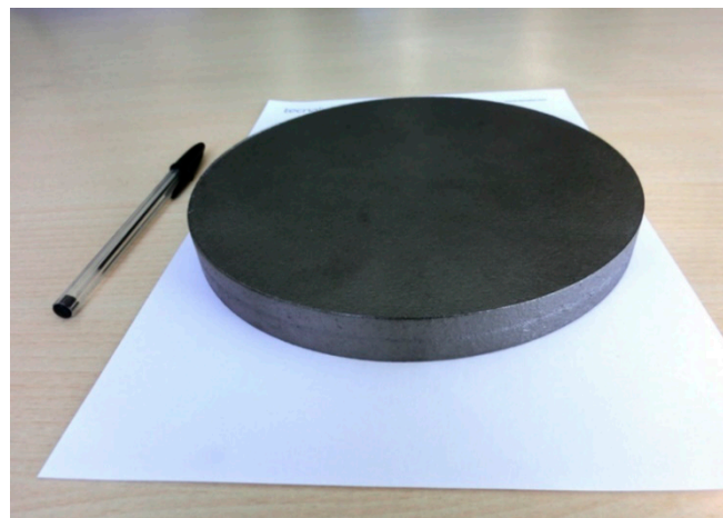
Figure 16. Ti composite part of large dimensions (20 cm in diameter), elaborated by SPS [95]. Reproduced with permission from Materials Science and Engineering: A , published by Elsevier, 2016.
