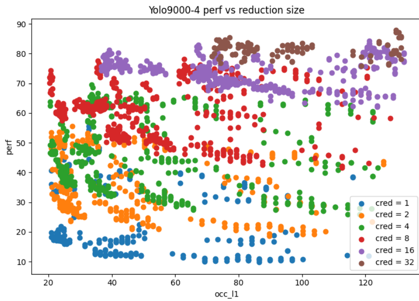
Figure 7: Exhaustive exploration of the optimisation space for Yolo9000-4, and classification according to the tile size of the reduction loop c above the \mu kernel and L1 cache occupancy.
