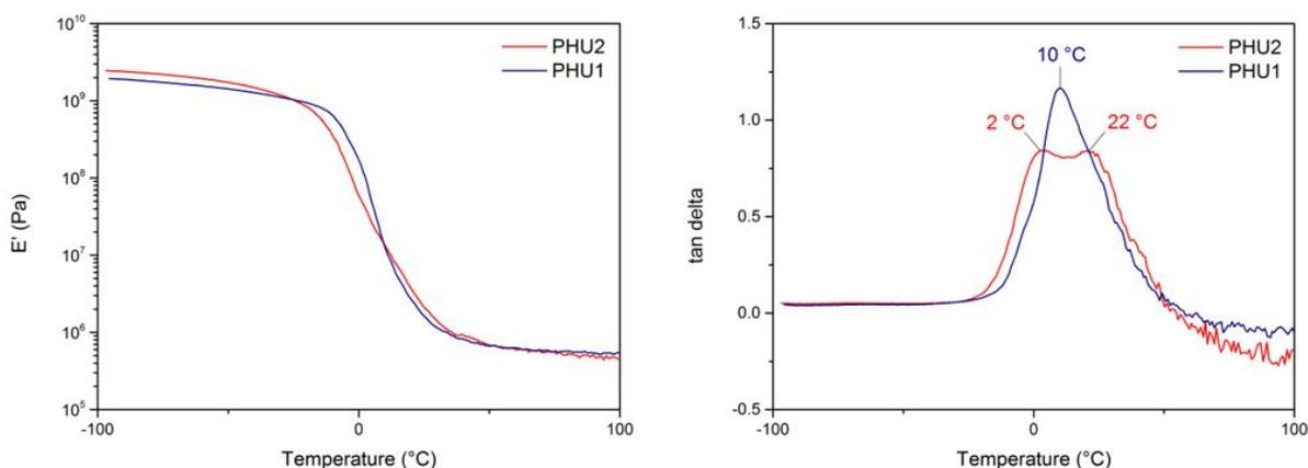
Figure 8: DMA measurements of PHU thermosets (right: storage modulus ( $E'$ ); left:  $\tan \delta$ ).
