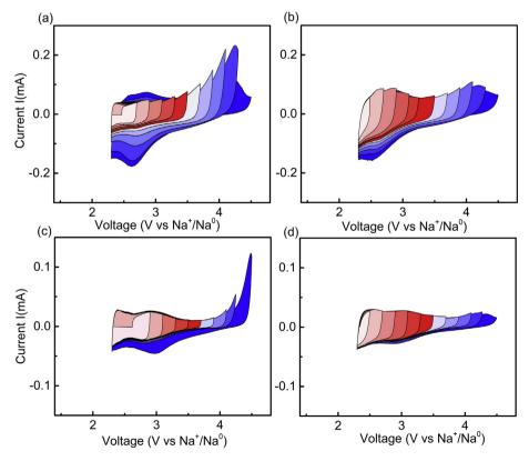
**Fig. 4.** Voltammetry technique through gradual enlargement of upper voltage limit up to 4.5V on (a, c) a new cell and (b, d) on a cell after 3 cycles vs.  $Na^+/Na^0$  in 3-electrode Swagelok type cell at scan rate of 0.05 mV/s for (a,b) sample P2– $Na_{0.72}$ [Mg<sub>0.31</sub>Mn<sub>0.69</sub>]O<sub>2</sub> and (c,d) sample P2– $Na_{0.63}$ [ $\Box_{0.036}$ Mg<sub>0.143</sub>Mn<sub>0.82</sub>]O<sub>2</sub> respectively.
