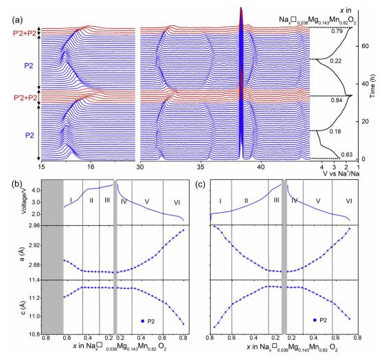
**Fig. 7.** (a) operando XRD patterns of P2 type  $Na_{0.63}[\Box_{0.036}Mg_{0.143}Mn_{0.82}]O_2$  upon 2 cycles as a function of Na amount at C/30 (The corresponding time versus voltage plot is shown on the right) and evolution of refined cell parameter  $a_{P2}$  and  $c_{P2}$  upon (b) first cycle and (c) second cycle.
