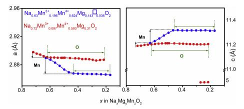
Fig. 8. Evolution of refined cell parameters a and c upon first charge with identification of redox domain for samples  $Na_{0.63}[\square_{0.036}Mg_{0.143}Mn_{0.82}]O_2$  and  $Na_{0.72}[Mg_{0.31}Mn_{0.69}]O_2$ .
