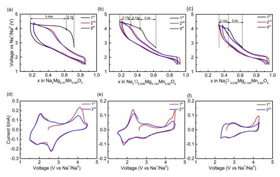
**Fig. 3.** (a) (b) (c) Voltage profile at C/20 at room temperature and (d) (e) (f) Cyclic voltammetry profile at scan rate of 0.05 mV/s for of P2–  $Na_{0.72}[Mg_{0.31}Mn_{0.69}]O_2$ ;  $Na_{0.63}[\Box_{0.036}Mg_{0.143}Mn_{0.82}]O_2$  in [1.5–4.5V] voltage range and  $Na_{0.63}[\Box_{0.036}Mg_{0.143}Mn_{0.82}]O_2$  in [1.5–4.5V] voltage range.
