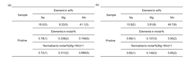
Table SI-1: Chemical composition analysis by ICP-AES for  $Na_xMg_yMn_{1-y}O_2$  with (a) y=0.3 and (b) y=0.15.
