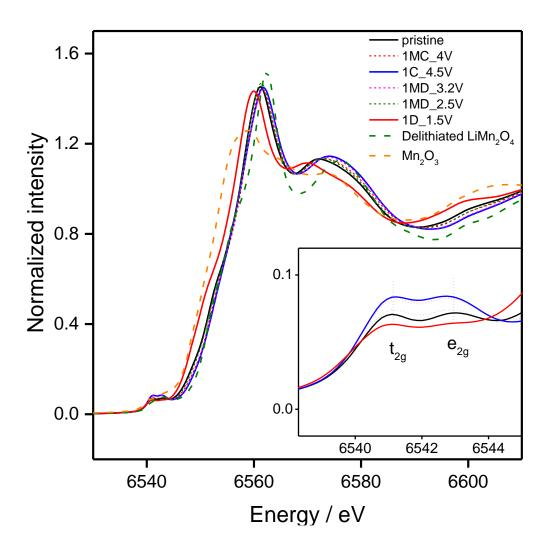
Figure SI-2: Mn K-edge XANES spectra of (a) *ex-situ* P2- Na<sub>0.72</sub>[Mg<sub>0.31</sub>Mn<sub>0.69</sub>]O<sub>2</sub> including pristine, mid-charged(4 V), fully charged(4.5 V), mid-discharged(3.2 V), mid-discharge (2.5 V) and fully discharged (1.5 V) states, compared with some selected references for Mn<sup>3+</sup> (Mn<sub>2</sub>O<sub>3</sub>) and Mn<sup>4+</sup> (LiMn<sub>2</sub>O<sub>4</sub> delithiated). The inset shows a zoom of the pre-edge region.
