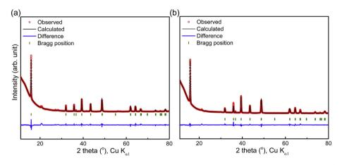
Fig. 2. Results of Rietveld refinement of XRD patterns of P2-type a) Na<sub>0.72</sub>[Mg<sub>0.31</sub>Mn<sub>0.69</sub>]O<sub>2</sub> and b) Na<sub>0.63</sub>[ $\Box_{0.036}$ Mg<sub>0.143</sub>Mn<sub>0.82</sub>]O<sub>2</sub> based on S.G. P6<sub>3</sub>/mmc.
