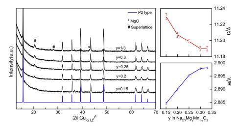
**Fig. 1.** (a) Evolution of XRD patterns of P2 type  $Na_{2/3}[Mg_yMn_1_y]O_2$  with y = 0.15, 0.2, 0.25, 0.3, 1/3 and calculated one using the structure data from P2 type structure. (b) Evolution of refined cell parameters *a* and *c* with the amount of Mg.
