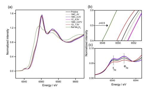
**Fig. 5.** (a) Mn K-edge XANES spectra of *ex-situ* Na<sub>0.63</sub>[ $\square_{0.036}$ Mg<sub>0.143</sub>Mn<sub>0.82</sub>]O<sub>2</sub> including pristine, mid-charged (4V), mid-charged (4.2V), fully charged (4.5V), mid-discharged (2.67V) and fully discharged (1.5V) states, compared with some selected references for Mn<sup>3+</sup> (Mn<sub>2</sub>O<sub>3</sub>). (b) zoom of the edge region, where Jump = 0.5 (c) zoom of the pre-edge region.
