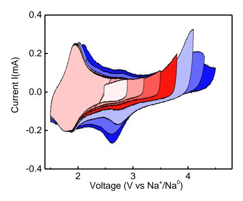
Figure SI-1: Cyclic voltammetry technique with gradual enlargement of upper voltage limit during the first cycle in the [1.5 or 2.3-4.5 V] vs. Na<sup>+</sup>/Na<sup>0</sup> voltage for P2-Na<sub>0.72</sub>[Mg<sub>0.31</sub>Mn<sub>0.69</sub>]O<sub>2</sub>. Data are collected in 3-electrodes Swagelok type cell at scan rate of 0.05mV/s.
