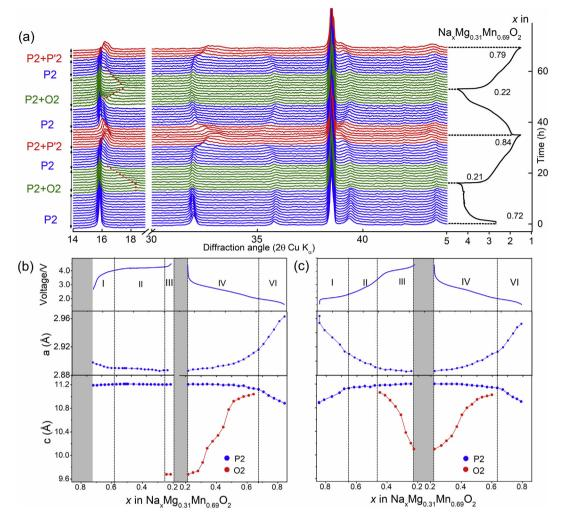
**Fig. 6.** (a) operando XRD pattern of P2 type  $Na_{0.72}[Mg_{0.31}Mn_{0.69}]O_2$  upon 2 cycles as a function of Na amount at C/30 (The corresponding time versus voltage plot is shown on the right) and evolution of refined cell parameter  $a_{P2}$  and  $c_{P2}$  upon (b) first cycle and (c) second cycle.
