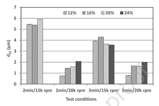
**Figure 2**: Determination of conditions of use of rotor stator system, BRSE, based on the formulation PCP (Table 2): variation of the Sauter diameter, d<sub>32</sub>, as a function of speed rotation of stator, duration of mixing and volume fraction of dispersed phase in emulsions (in %).
