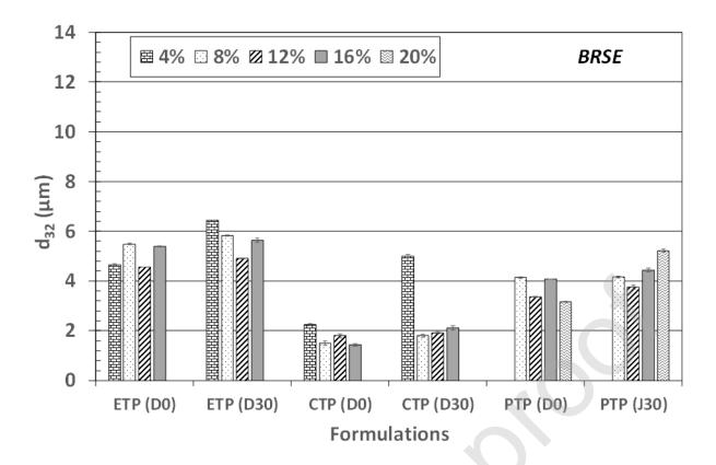
**Figure 7**: Comparison of the values of the Sauter diameter corresponding to fresh emulsions (D0) and emulsions after 30 days of storage (D30). Emulsions were obtained with ETP, CTP and PTP formulations using BRSE. The volume fraction of the dispersed phase is indicated in %. All trials have been repeated twice (the scatter is indicated with an error bar).
