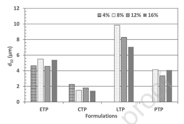
**Figure 3**: Sauter diameter, d<sub>32</sub>, (in μm) obtained with 4 formulations (see Table 2) and various oil fractions (in %) after 5 min. at 15,000 rpm using the BRSE.
