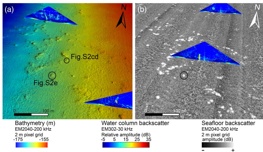
**Figure 2.** The 3-D views of a seeping area at the Aquitaine Shelf edge (Figure 4). Processed polar echograms of the water column are superimposed on high-resolution (a) shaded bathymetry and (b) seafloor backscatter. The seafloor is densely populated with carbonate mounds characterized by high-amplitude seafloor backscatter. Among the 161 seeps evidenced by water column acoustics in this area, a few tens of them were investigated during the GZ2-ROV535 dive (Figure S2).
