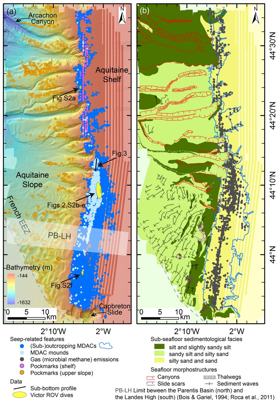
**Figure 4.** Detailed (a) shaded bathymetric and (b) subseafloor sedimentological maps of the Aquitaine Shelf edge area with indication of methane emissions, seep-related features, and seafloor morphological structures.
