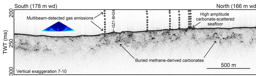
**Figure 3.** Subbottom profile across seeping sites at the Aquitaine Shelf edge (Figure 4a). Grab sampling along this profile (GZ1-BH24) recovered authigenic carbonates (Pierre, Demange, et al., 2017). Gas emissions, along the profile and within its close vicinity (less than 20 m), are reported.
