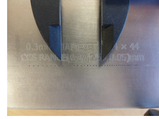
Fig. 10. Stainless steel block containing a set of 41 close aligned SDHs ( \varnothing 0.3 mm), with decreasing distance from left to right.
