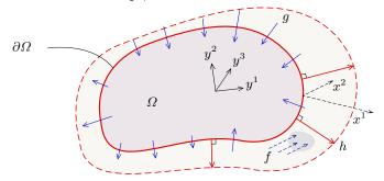
Figure 3: A submanifold  $\Omega$  described by local coordinates  $y^1, \ldots, y^n$  and parameterised over codimensions  $x^1, \ldots, x^m$ . The physical flux in the plane of  $\Omega$  corresponds to the (m+n-1)-form g and the pseudo flux, arising from the normal flux f through deformations in  $\partial \Omega$  as one moves with unit 'velocity' in the direction  $x^i$  corresponds to the (m+n-1)-form h.
