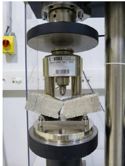
Fig. 5. Flexural test.
