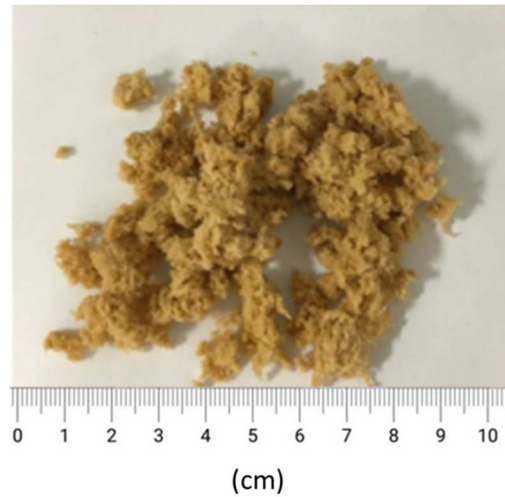
Fig. 1. Wastes of VSS after grinding, washing and drying.
