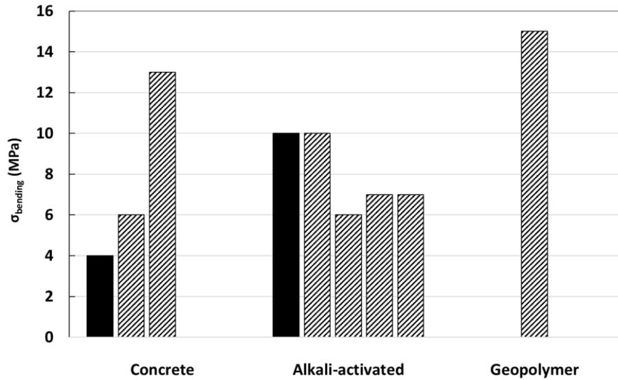
**Figure 7:** bending values in the literature for concretes (Wolf et al. 2019, Bos et al. 2019, Le et al. 2012), alkali-activated materials (Paul et al. 2018, Bong et al 2019, Al-Qutaifi et al 2018, Panda et al. 2017, Korniejenko et al. 2019) and geopolymers (values from this study) for ■ binders and ▨ composites shaped by robocasting.
