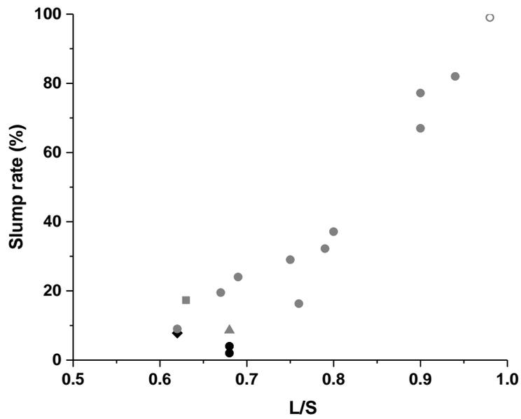
**Figure 3:** slump rate as function of the ratio L/S for the formulations shaped with the robocasting process ( $v_z = 62 \cdot 10^{-6}$  m/s) with (○) the M<sub>16</sub> binder and the (●) M<sub>16</sub>W<sub>a</sub>G<sub>b</sub>, (▲) M<sub>19</sub>W<sub>10</sub>G<sub>2</sub>, (■) M\*W<sub>21</sub>G<sub>2</sub>, (●) M<sub>16</sub>W<sub>a</sub>G<sub>b</sub>A<sub>c</sub>Ki<sub>d</sub> and (◆) M<sub>16</sub>W<sub>21</sub>G<sub>2</sub>Sa<sub>6</sub> composites (see Table 2).
