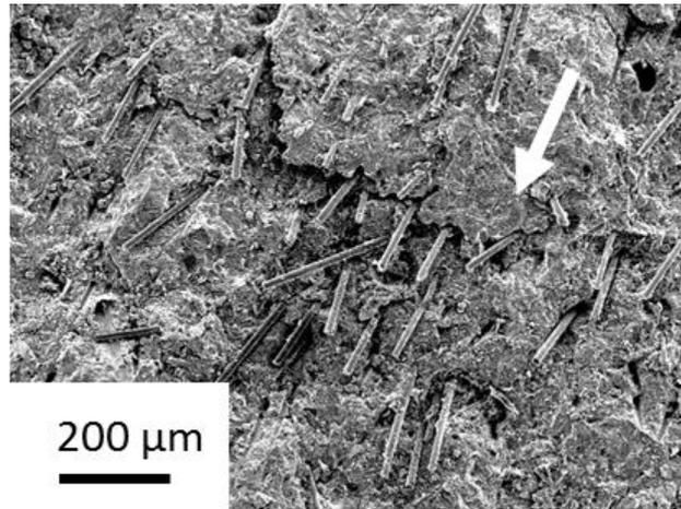
**Figure 6:** SEM photos of the microstructure of M<sub>16</sub>W<sub>10</sub>G<sub>2</sub> geopolymers shaped by robocasting (↗ represent the printing direction).
