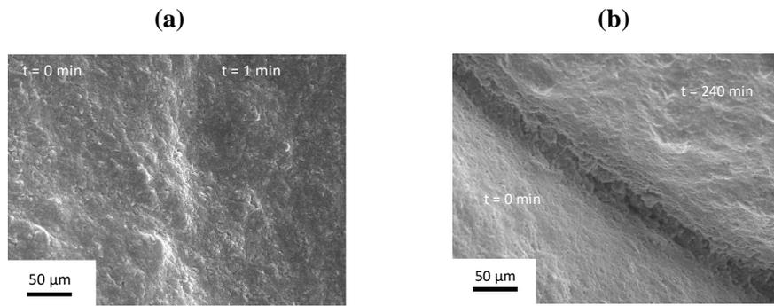
**Figure 4:** SEM photos of the interface between two fresh layers of a geopolymer M<sub>19</sub> extruded with a syringe ( $\Phi_{\text{buse}} = 2 \text{ mm}$ ) with a time gap of (a) 1 and (b) 240 minutes.
