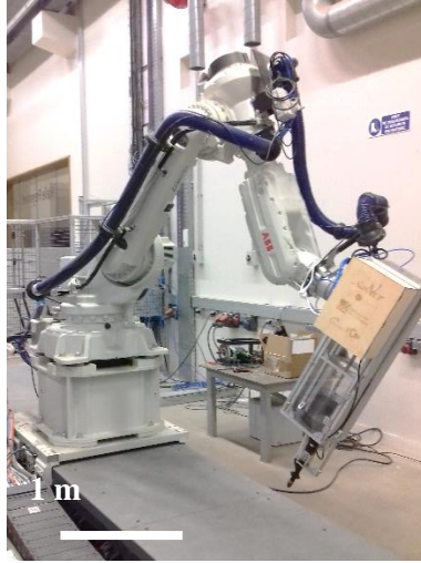
Figure 8: a geopolymer own-developed extruding tool mounted on a 6-axis robot (Build'In platform).
