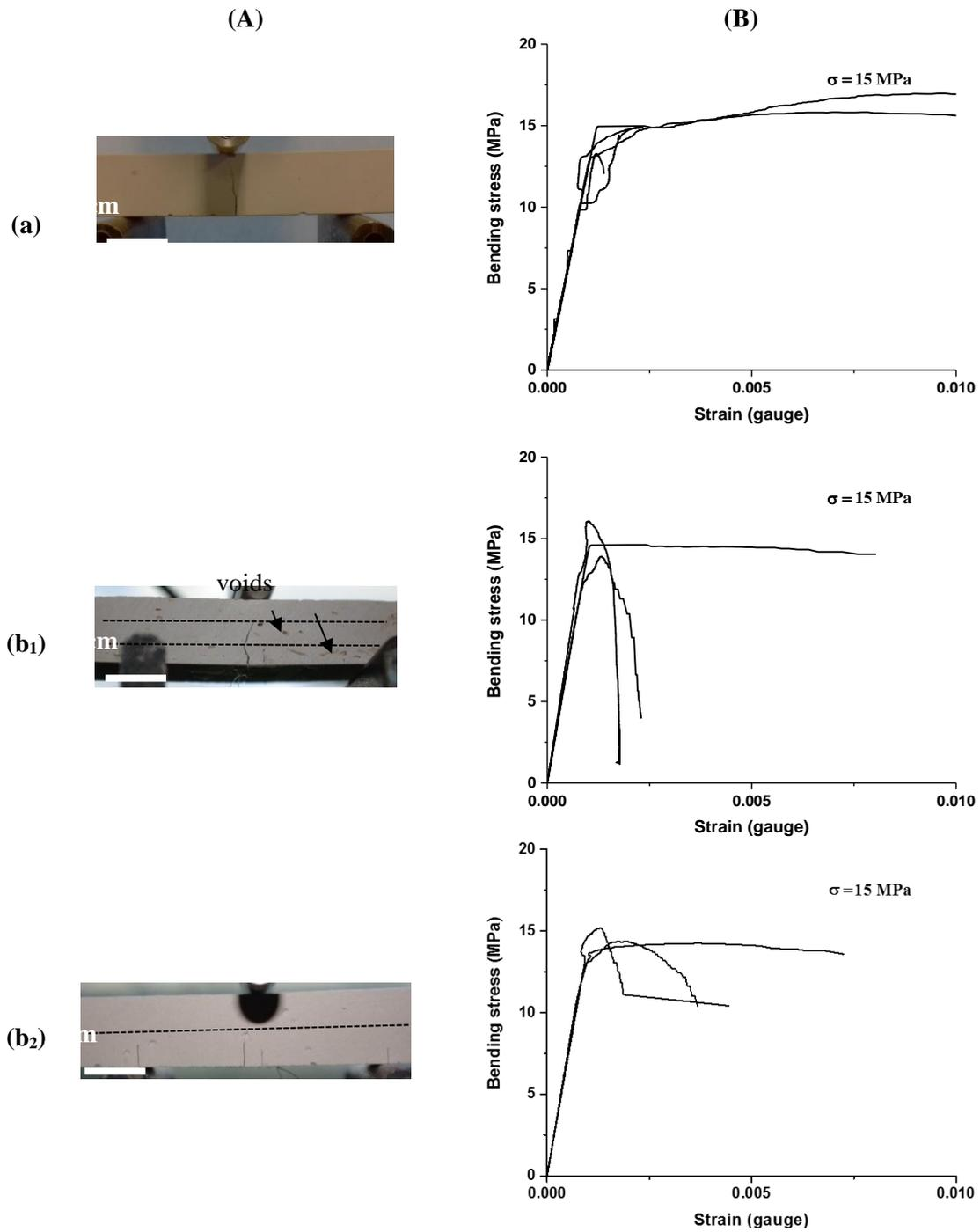
**Figure 5:** (A) photos after failure and (B) axial stress as a function of strain for the 3-points bending samples elaborated by (a) casting and by robocasting in (b<sub>1</sub>) perpendicular and (b<sub>2</sub>) lateral directions (see Figure 1).
