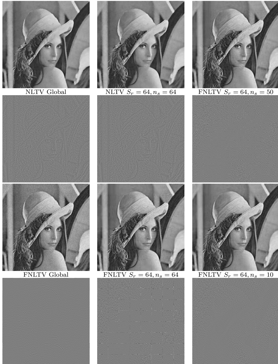
FIGURE 12. Left: image denoised by NLTV and FNLTV globally; Middle: image denoised by NLTV and FNLTV locally with no-overlapping regions of size 64 \times 64 ; Right: image denoised by NLTV and FNLTV locally with overlapping regions of size 64 \times 64 for moving step n_s = 50 (top) and n_s = 10 (third row). The second and bottom rows are the method noise images of the corresponding images of the top and third rows.
