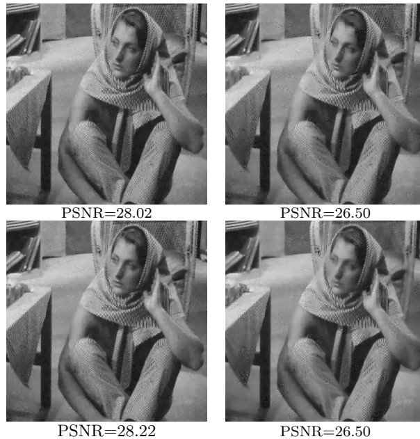
FIGURE 8. Left: image denoised by choosing \lambda with smallest estimated MSE; right: choosing \lambda randomly. Top: region size 16 \times 16 ; bottom region size 32 \times 32 .
