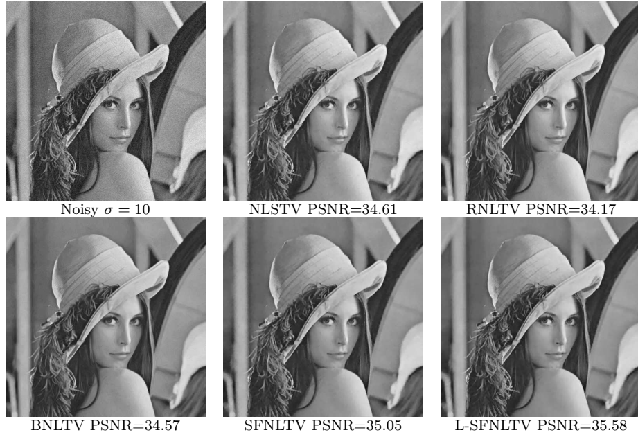
FIGURE 16. Denoised Lena images by L-SFNLTV, NLSTV [15], RNLTV [17], BNLTV [18] and SFNLTV in the case \sigma = 10 .
