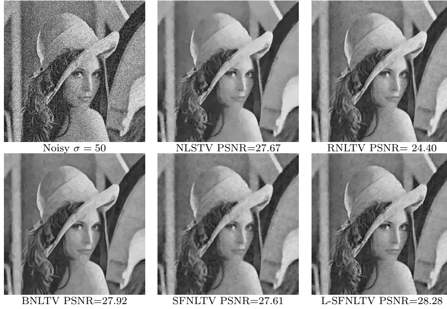
FIGURE 18. Denoised Lena images by L-SFNLTV, NLSTV [15], RNLTV [17], BNLTV [18] and SFNLTV in the case \sigma = 50 .
