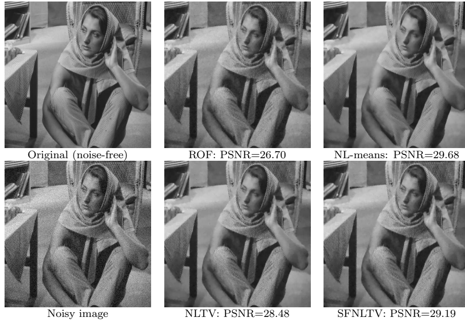
FIGURE 14. Denoised images by ROF model, NL-means, NLTV model and SFNLTV model for Barbara.
