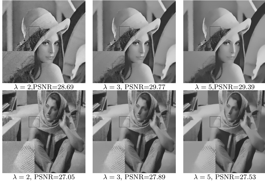
FIGURE 5. Denoised image by NLTV with D = 11 for different values of \lambda with \sigma = 20 .
