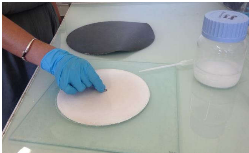
Figure 41 : Grinding and polishing of a thin slice of otolith
