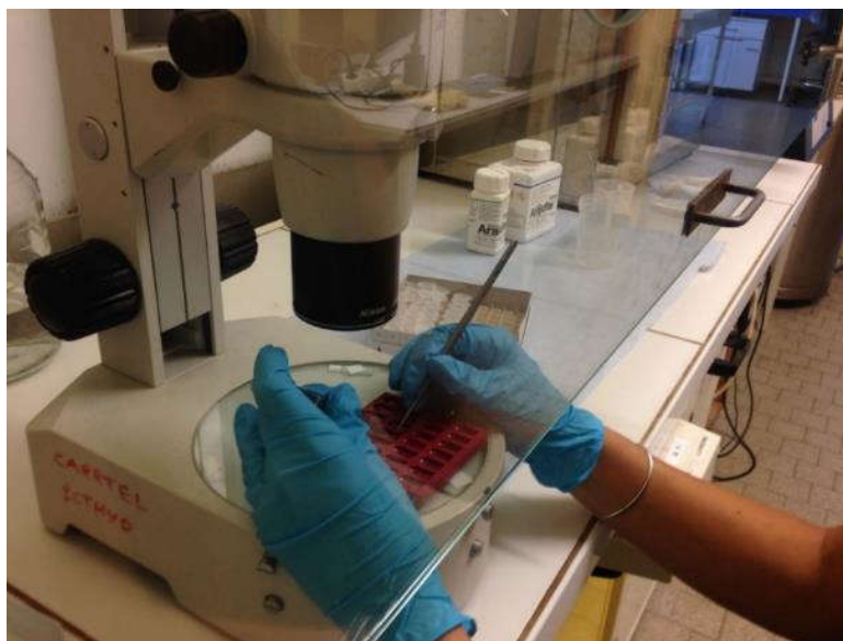
Figure 39 : Otolith positioning in molds under a dissecting microscope
