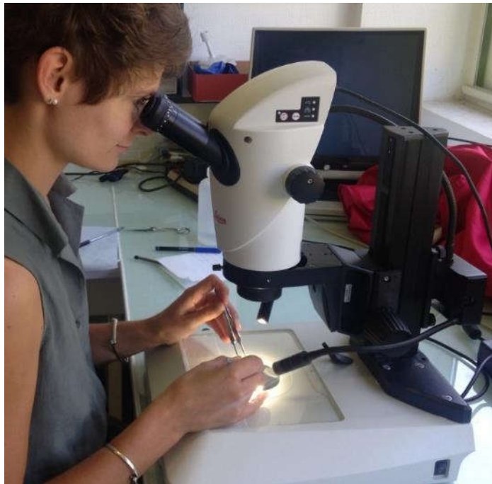
Figure 36 : Otolith photography under LEICA dissecting microscope
