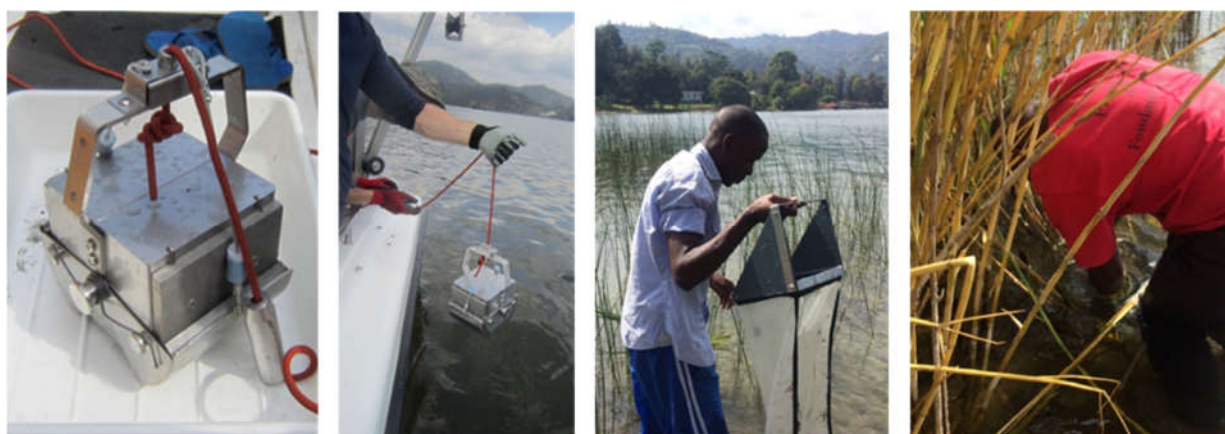
Figure 12 : Sampling using Ekman sediment trap and Sürber net
