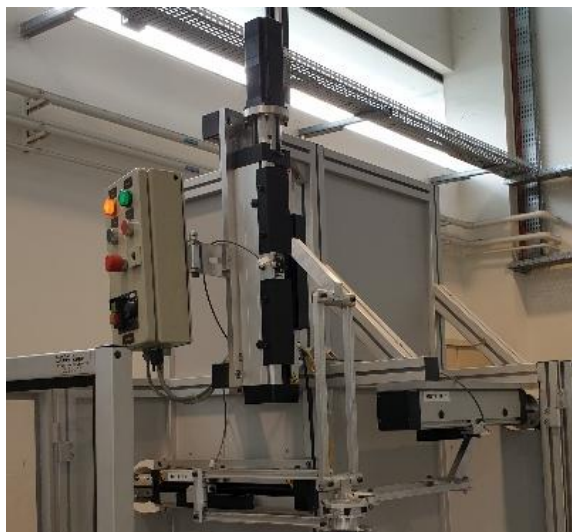
Figure 2. The prototype of the Orthoglide (LS2N).
