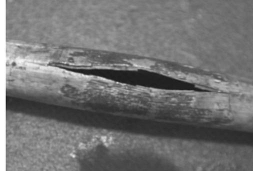
Fig. 16. Burst test on ZIRLO sample (DFIM).
