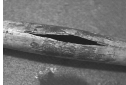
Fig. 16. Burst test on ZIRLO sample (DFIM).
