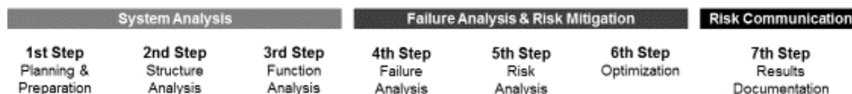
Figure 3. The 7-step FMEA approach (AIAG and VDA 2019)
