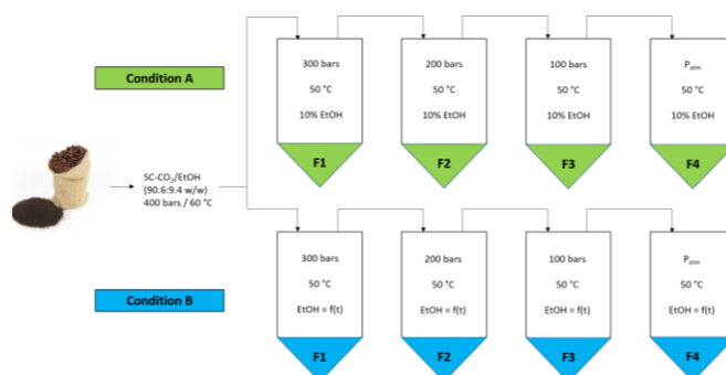
Figure 11: Fractionation process of SC-CO 2 extraction of SCG for production of extracts enriched in phenolic compounds, adapted from Bitencourt et al. 196
