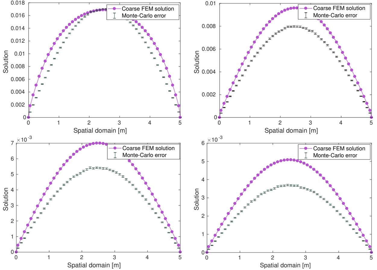
Figure 1: Coarse finite element resolution and statistical Monte Carlo error at time step  $n = 1$  (top left),  $n = 3$  (top right),  $n = 4$  (bottom left), and  $n = 5$  (bottom right).
