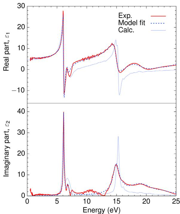
**Figure 1.** Real (upper panel) and imaginary (lower panel) ordinary dielectric functions of *h*-BN. The dotted lines represent model fits to the data. The point-by-point fits to the experimental ellipsometric data (red lines) are compared with the results of ab initio calculations (light blue curves).
