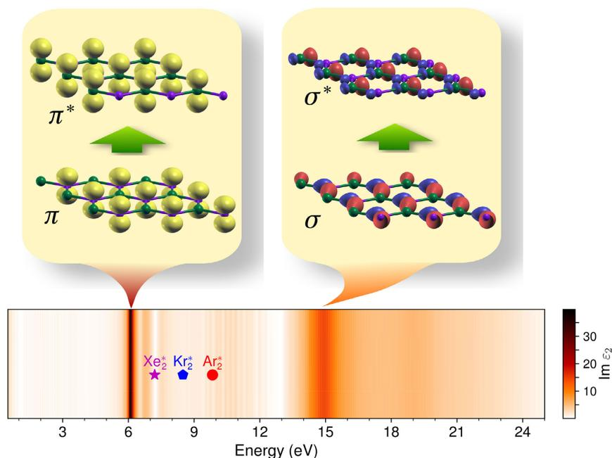
**Figure 4.** Transparency window in  $h$ -BN between the fundamental bandgap absorption driven by  $\pi \rightarrow \pi^*$  transitions and the higher bandgap absorption driven by  $\sigma \rightarrow \sigma^*$  transitions. The symbols indicate the emission energies of the most commonly used deep-UV excimer lamps (from ref. [11]). In the sketch of the orbitals, green balls represent boron atoms and purple balls represent nitrogen atoms.
