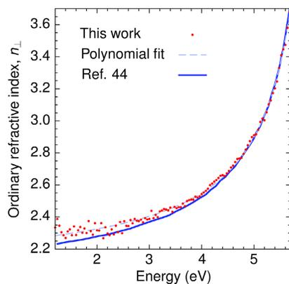
**Figure 2.** Below-bandgap ordinary refractive index of *h*-BN derived from ellipsometric measurements compared with previous optical transmittance determination. The dashed line is a rational polynomial fit to the ellipsometric data.
