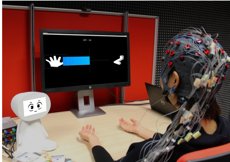
Figure 1: A participant training to perform mental tasks on the right with PEANUT, the first learning companion dedicated to MI-BCI user training, on the left.
