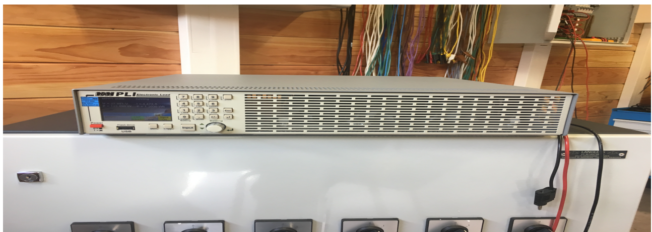
Figure 10: Device for PV module characteristics measurement.
