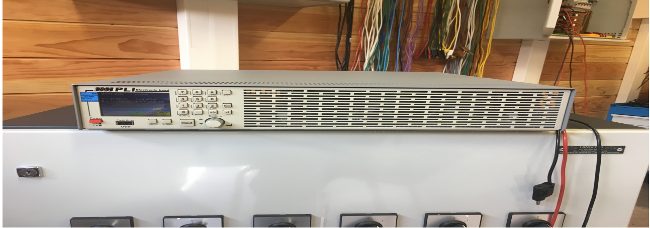
Figure 10: Device for PV module characteristics measurement.
