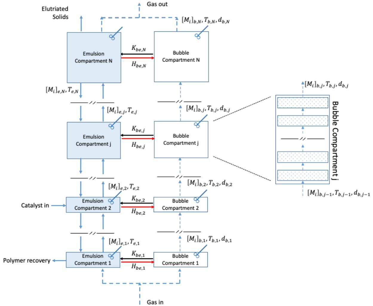
Figure 10. Concept of the fully compartmentalised model.
