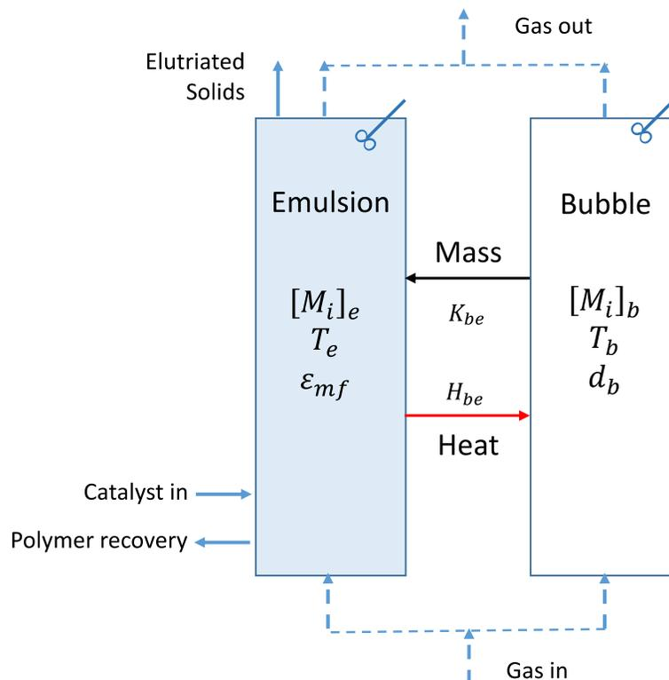
Figure 6. Two-phase constant bubble size model. Each compartment is treated as a CSTR. The symbols are defined in the text.
