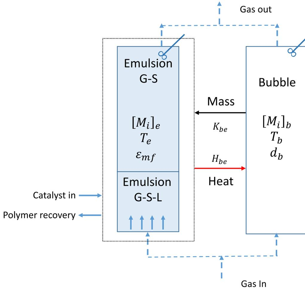
Figure 7. Two-phase model of Zhou *et al.* [115]. The emulsion phase is divided in a gas-solid-liquid (G-S-L) region at the bottom that moves from the distributor plate to the next zone via plug flow and in a gas-solid (G-S) upper region which is well-mixed. The bubble phase is a well-mixed zone.
