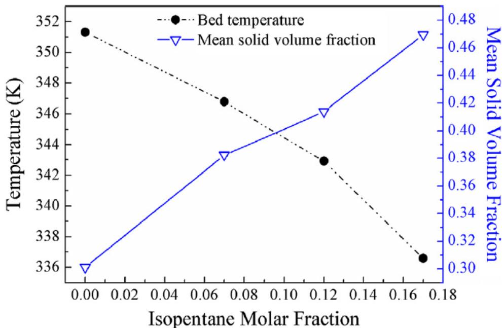
Figure 13. Mean bed temperature and solid volume fraction as a function of the molar fraction of isopentane. Reproduced with permission from Pan *et al.* [157] Copyright 2016 The Society of Powder Technology Japan.
