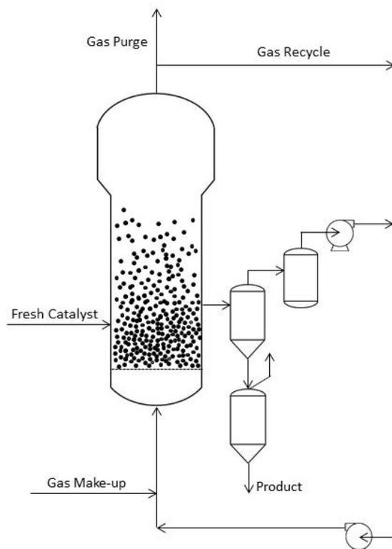
Figure 1. Scheme of typical fluidized bed reactor.
