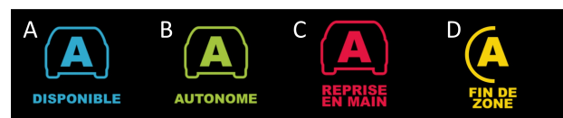
Figure 2: Pictograms displayed on the HMI. A: autonomous driving available; B: autonomous driving activated; C: take-over request (8 s); D: take-over request (45 s)
