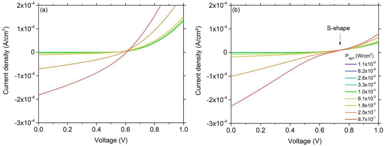
FIG. 4. Current density under illumination with different intensities from  $1.1 \times 10^{-6} \text{ W/cm}^2$  to  $8.7 \times 10^{-1} \text{ W/cm}^2$  for the devices processed with PEDOT:PSS (a) and p-doped PBDTTT-c (b) as HTL. The arrow indicates the S-shape formed around  $V_{OC}$  at higher light for the device with p-doped polymer as HTL.
