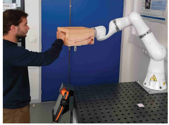
Fig. 1. Human robot collaboration to move a box with the robot Kuka LBR iiwa 14 R820.
