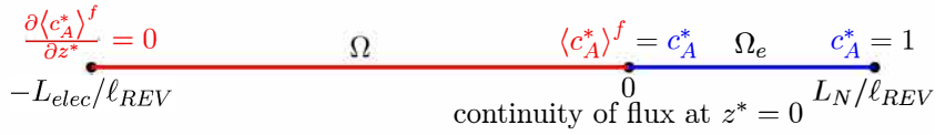
Fig. 5.1. Configuration of the 1D domain including the electrode ( \Omega ) and Nernstian layer ( \Omega_e ).
