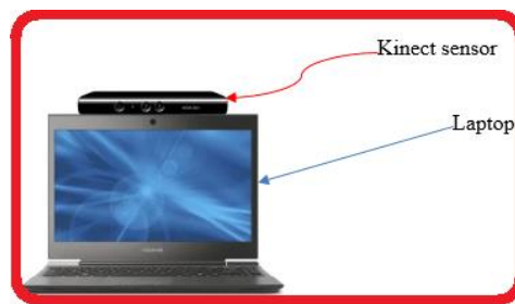
Figure 30. Acquisition environment for the Kinect face database.
