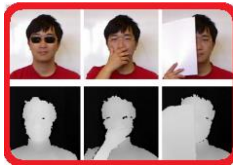
Figure 36. Occlusions by sunglasses, by hand and by paper. Upper: the RGB (red green blue) images. Lower: the depth maps aligned with above RGB images.
