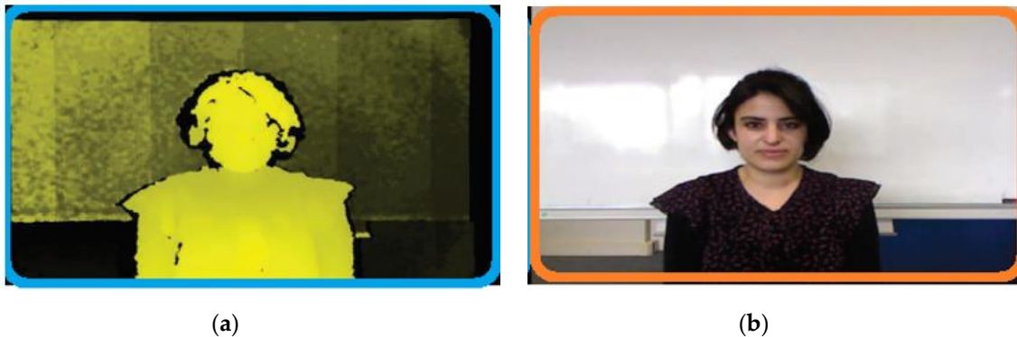
Figure 31. RGB-D (red green blue-depth) alignment: (a) the depth map is aligned with (b) the RGB image captured by Kinect at the same time.
