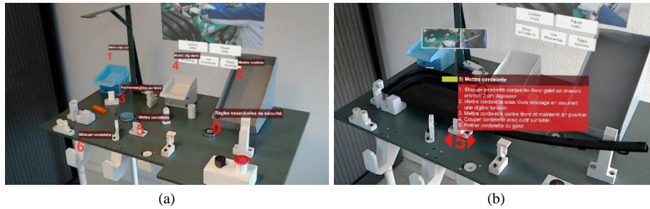
Fig. 2. Screenshots of the training application in AR mode: (a) Overview of the assembly task, (b) WI details of a specific step, plus added contents.
