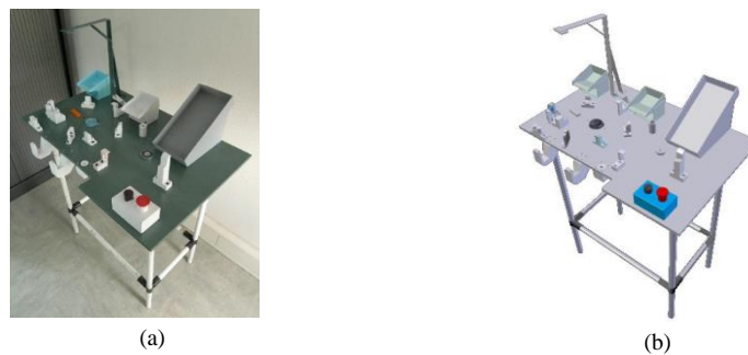
Fig. 1. The Finishing table : (a) the physical prototype and (b) its digital mock-up.
