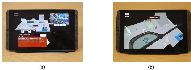
Fig. 3. Tablet prototype: (a) Initial training screen. Note the decomposition of the UI in dedicated zones for animations, videos, textual instructions, and additional images, (b) full-screen 3D view, which can be manipulated freely.
