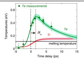
FIG. 4. Time evolution of both electron  $(T_e)$  and ion  $(T_i)$  temperatures estimated with the two-temperature code at  $F_{abs} = 0.065 \pm 0.015 \text{ J/cm}^2$  (see details in the text), and convoluted with the time instrumental response. The shaded areas come from the fluence uncertainty. Values of  $T_e$  deduced from the pre-edge measurements are reported (circles).
