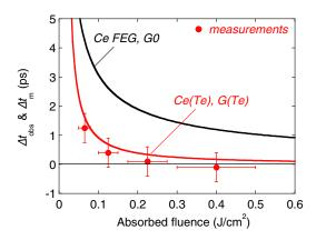
FIG. 5. Time delay  $\Delta t_{obs}$  for the electron structure transition from fcc to liquid, measured as a function of the absorbed laser fluence. Data are compared with two-temperature calculations performed with two sets of physical parameters ( $\Delta t_m$ , see details in the text).
