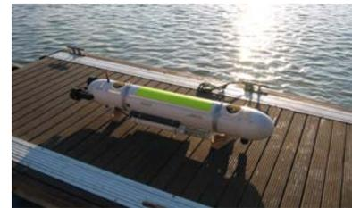
Fig. 2. Modular Autonomous Robot for Environment Sampling [2].
