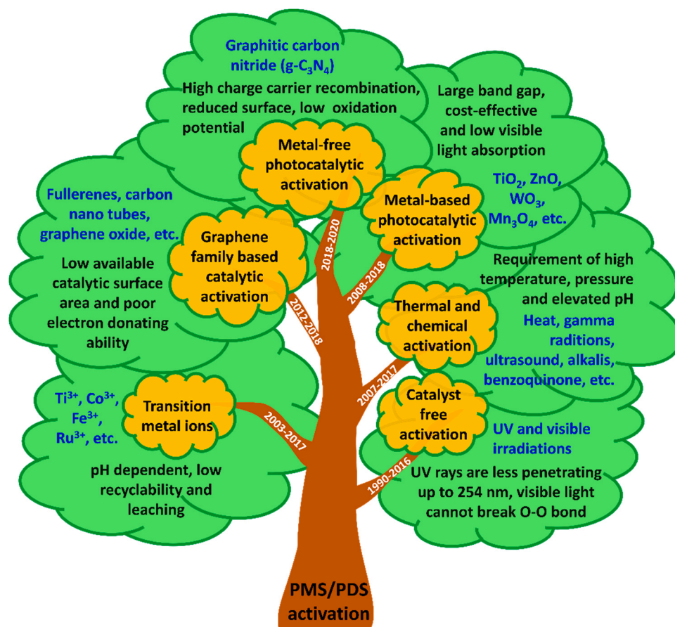
Fig. 1. Evolution tree of peroxymonosulfate/ peroxydisulfate (PMS/PDS) activation methods with their respective disadvantages.
