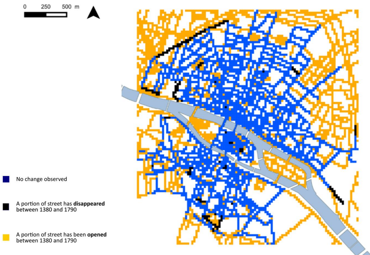
Figure 1. Comparison of two maps (1380 and 1791) of the Parisian street network through an analysis grid (squares of 25x25 m). © Léa Hermenault
