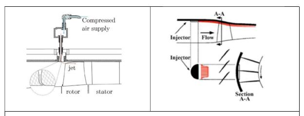
**Figure 3.** Two examples of tip blowing experiments in axial compressor, from [3] (left) and [8] (right).
