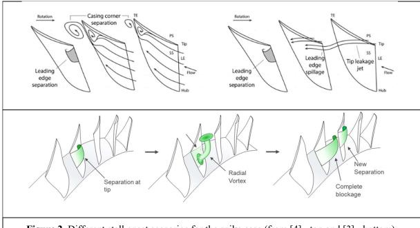
Figure 2. Different stall onset scenarios for the spike case (from [4] - top and [3] - bottom).
