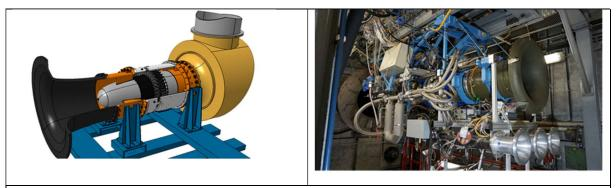
**Figure 6.** Test benches used in ACONIT project: CME2 single stage axial compressor (left) and Larzac turbojet engine (right).
