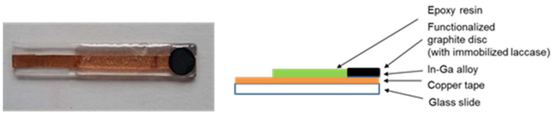
Figure 2. Photograph and schematic of the biocathodes developed in this work
