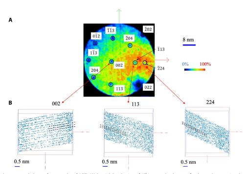
**Fig. 4. Analyzing aluminum nanotip in terahertz-assisted APT.** (**A**) Spatial distribution of Al<sup>+</sup> ions on the detector for the terahertz-assisted atom probe analysis. (**B**) 3D images resulting from the terahertz-assisted atom probe analysis showing Al atomic planes along the <002>, <113>, and < 224> crystallographic directions; black dotted lines are guides to the eye.
