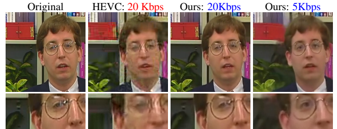
Fig. 3: Qualitative evaluation against HEVC on Deadline (Frame 40) sequence in a low bitrate setting.
