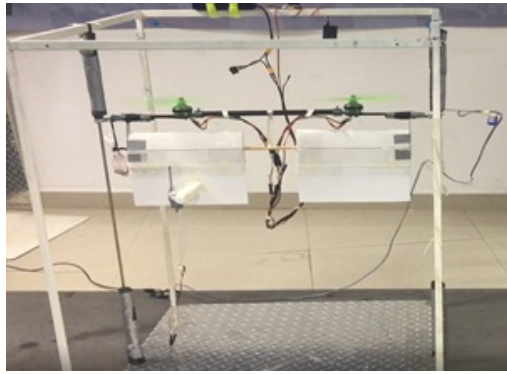
(a) Test bench to studied the airstream generated by the rotors.
