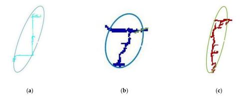
**Figure 6.** Misidentification of connected components (CCs) using existing edge detection methods. (a) Joining horizontal and vertical architectural lines and (b,c) joining architectural lines and cracks.
