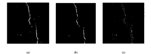
**Figure 4.** Performance of edge detection operators on rammed earth images. (**a**) Sobel, (**b**) Prewitt and (**c**) Laplacian of Gaussian.
