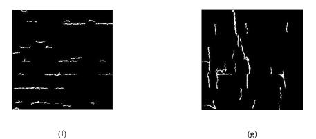
**Figure 14.** Evaluation of the algorithm on surface images of earthen heritage. (**a**) Image 1, (**b**) horizontal edge map, (**c**) vertical edge map, (**d**) horizontal CCs (area > 30 pixels), (**e**) vertical CCs (area > 30 pixels), (**f**) architectural feature map and (**g**) crack map.
