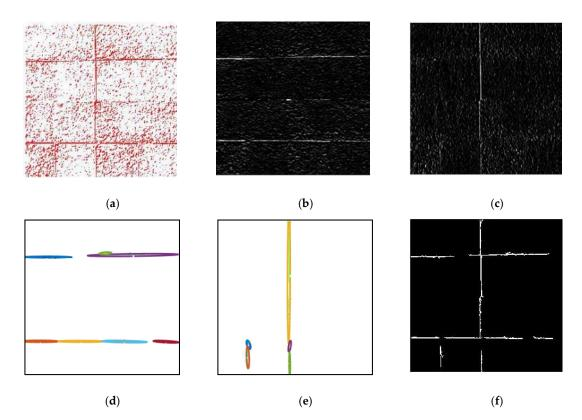
**Figure 17.** Evaluation of algorithm on surface images of earthen heritage. (**a**) Image 4, (**b**) horizontal edge map, (**c**) vertical edge map, (**d**) horizontal CCs (area > 30 pixels), (**e**) vertical CCs (area > 30 pixels) and (**f**) architectural feature map.
