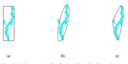
Figure 8. Morphological parameters. (a) Bounding box, (b) bounding ellipse and (c) convex hull.
