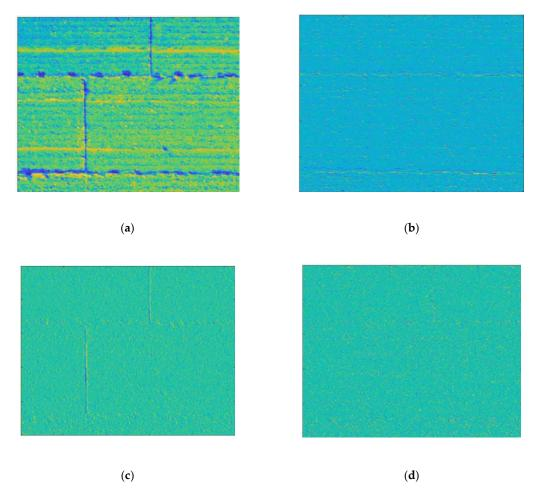
**Figure 5.** Sub-bands obtained by Haar transform on a rammed earth image. (**a**) Approximate edge map, (**b**) horizontal edge map, (**c**) vertical edge map and (**d**) diagonal edge map.
