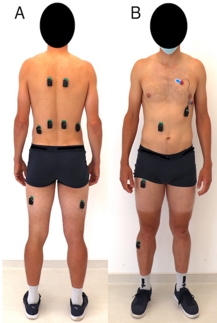
Figure 9 - ECG and surface EMG placement for the quantification of Laevo's assistance during a PP maneuver. A: EMG sensors on ESL, ESI, TA, BF and GM. B: ECG sensor with 2 electrodes and EMG sensors on RA, RF and TA.
