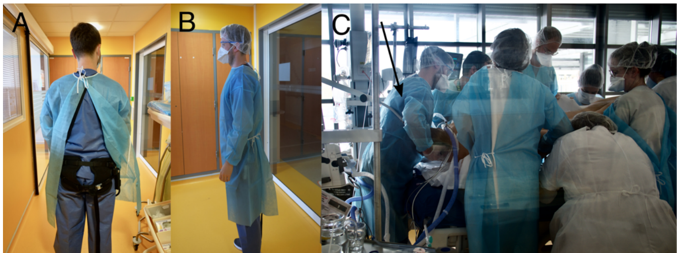
Fig. 7. Laevo used in the ICU. A and B: the exoskeleton is worn on clothes, hidden below the medical gown. C: the exoskeleton assists the physician positioned behind the head of the patient during a PP maneuver.
