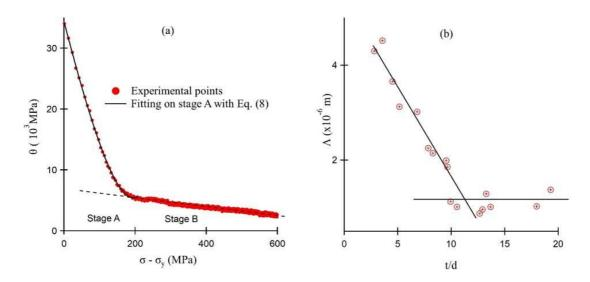
**Figure 15** – (a) Modeling of the work hardening curve of cobalt by using Eq. (8) (t/d = 13). (b) Evolution of the mean free path of dislocations in stage A with the t/d ratio for cobalt specimens of thickness 500  $\mu$ m.
