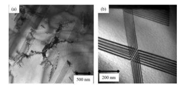
Figure 3 – Stacking faults observed in (a) hcp and (b) fcc phases of unstrained cobalt.
