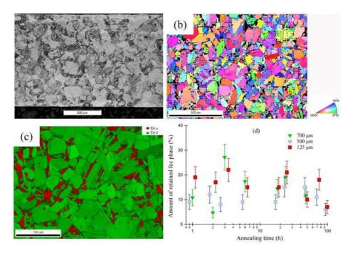
**Figure 1** – General overview of the microstructure of cobalt, unstrained state. (a) Grain size across the thickness, SEM, t/d = 14. (b) EBSD IPF map of the hcp phase, t/d = 14. (c) Cartography representing in red the hcp phase and in green the fcc one (t/d = 19). (d) Amount of residual fcc phase with the holding time of annealing at T = 1100 °C, for three thicknesses of cobalt samples.
