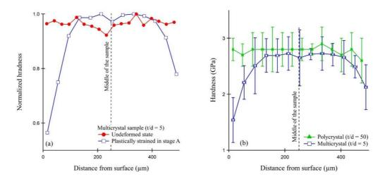
Figure 13 – (a) Normalized hardness values through the thickness of a multicrystal sample not deformed and strained in stage A. (b) Hardness profiles through the thickness of polycrystalline and multicrystalline samples plastically strained in stage A ( $t = 500 \mu m$ ). Errors bars in Fig. 13(a) are of the same order of magnitude than in Fig. 13(b).
