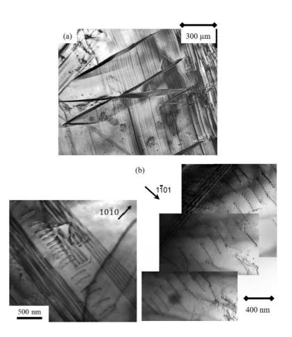
**Figure 10 –** Microstructural features of gliding mechanisms in cobalt. (a) Slip lines against twins in the beginning of plastic strain, confocal microscopy observation of a multicrystal. (b) Two examples of dislocation pile-ups representative of slip mechanisms in stage A of cobalt polycrystals.
