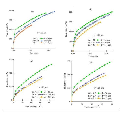
**Figure 4** – Typical true stress - true strain curves obtained in cobalt with various t/d ratio and a thickness of (a) 700  $\mu$ m, (b) 500  $\mu$ m, (c) 250  $\mu$ m and (d) 125  $\mu$ m.
