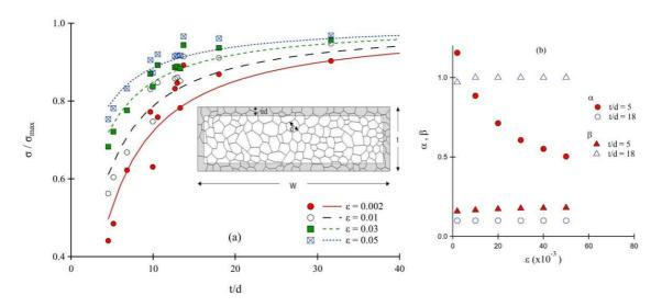
**Figure 14** – (a) Evolution of stress with t/d ratio for various plastic strains and corresponding analytical composite model (t = 500  $\mu$ m). In the inset: section of a rectangular flat tensile sample with corresponding geometrical parameters, following Shin and co-workers [69]). (b) Parameters  $\alpha$  and  $\beta$  in function of the plastic strain for a multicrystal (t/d = 5) and a polycrystal (t/d = 18)
