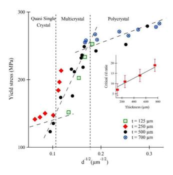
**Figure 8** – Initial HP plots for four distinct thicknesses showing the existence of the three crystalline configurations. In inset, evolution of the critical *t/d* ratio between multicrystalline and polycrystalline stages in function of the thickness.
