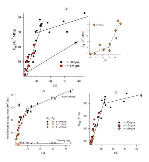
**Figure 9** – Evolution of the hardening parameters with t/d ratio computed from Fig. 5. (a) Initial work hardening rate  $\theta_0$ , (b) absolute values of slopes  $\Delta$  in stages A and B, (c) stress transition  $\sigma_{AB}$  between stages A and B.
