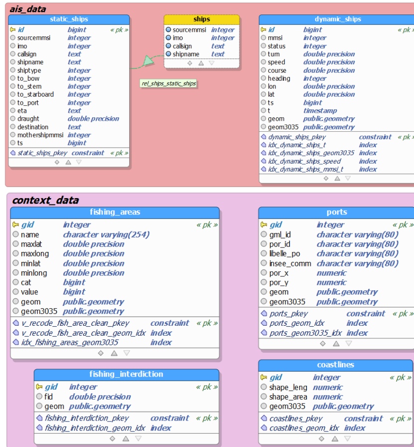
Fig. 13 Entities' structure (tables and views) of the database schemas ais_data and context_data . The data model is extracted from the PostgreSQL maritime database using pg-Modeler . 26
