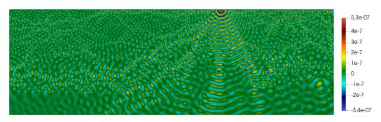
Figure 2: The real part of the solution to the Marmousi problem at a frequency of 20 Hz.
