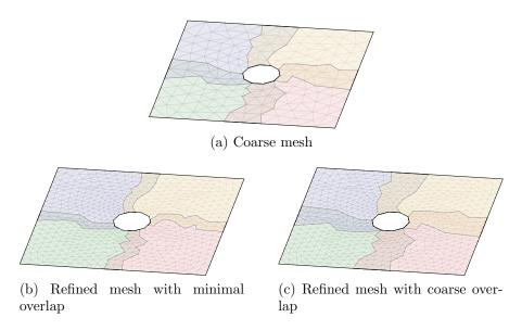
Figure 1: Different overlap definitions (bottom) for a uniformly refined simple 2D coarse mesh (top).
