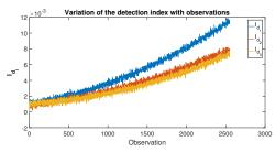
Figure 7: Variation of the detection indices (Degraded network without abrupt soft fault).
