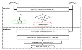
Figure 2: Fault detection and localization algorithm.
