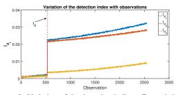
Figure 8: Variation of the detection indices (Degraded network with the appearance of a soft fault at  $t_0$ ).
